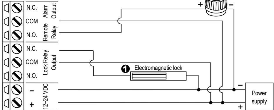
1. An electromagnetic lock, such as the E-941SA-1200, is connected to the lock relay output.
